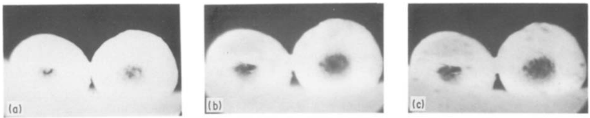
Figure 5 Spheres of \alpha -Al 2 O 3 single crystal sintered at 1550°C for (a) 119 h, (b) 183 h and (c) 206 h. Radii of spheres are 1.7 \times 10^{-4} m.
