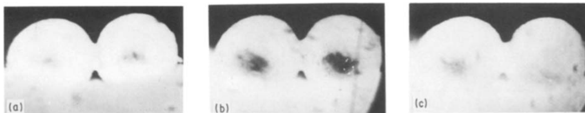
Figure 4 Spheres of MgO single crystal sintered at 1500^\circ\text{C} for (a) 50 h, (b) 143 h and (c) 213 h. Radii of spheres are 2.2 \times 10^{-4} m.
